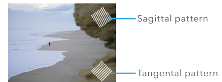
Examples of tangential and sagittal type patterns at the corners of the image.
