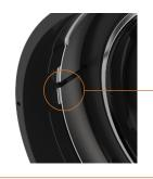
Before mounting a lens ensure the plastic collar supplied with the lens is in position and the joint is aligned with the location lug.
