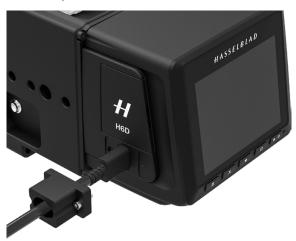
Attach the lock part and tighten the screws using the supplied 1.5mm Allen key. Note that it needs to be oriented correctly to fit.
