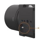
To detach the lens, press the lens release button on the side of the camera and turn the lens anti-clockwise.
